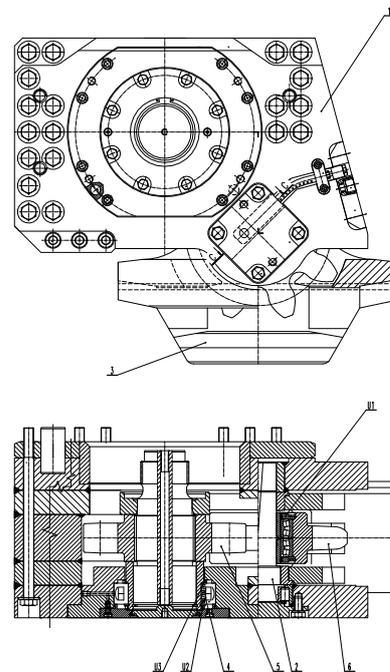
**Fig. 2.** Right (left) advance mechanism of the KSW-460NE type shearer:
