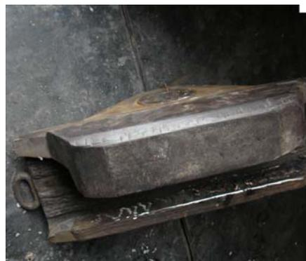
**Fig. 3.** Used and partially reconditioned guiding of the KSW-460 type shearer
