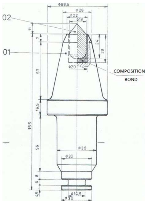
**Fig. 1.** Cutting tool for the KSW-460NE type shearer
